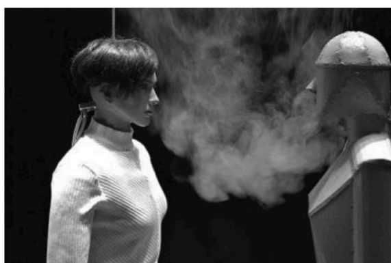
Fig. 2c. Smoke visualisation of exhalation flow from nose of the mannequin on the right – separation of mannequins was 0.4 M. The breathing zone of the mannequin on the left is again penetrated but its closer proximity to the exhaled smoke would suggest a greater degree of breathing zone penetration [14].
