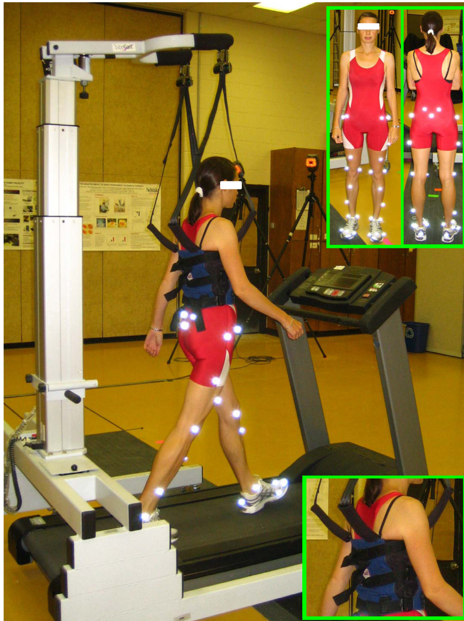
Figure 1 Experimental set-up with a subject fitted into the LiteGait ® system (Mobility Research, Inc., Tempe, AZ). This safety system consists of a lightweight waist harness straps linked to a telescoping metallic arm. The metallic arm was adjusted based on the subject's height so that the system did not provide any body weight support (slack straps). The absence of support was also monitored using the BiSym digital microprocessor of the LiteGait ® system. The harness size (small, medium and large) was selected based on the subject's upper body dimensions. It was tightened using locking straps located in the subject's back based on two criteria: (i) the subject had to feel comfortable wearing the harness while walking, and (ii) the harness had to fit well the waist without moving around it during walking. Reflective markers were attached to anatomical landmarks on the lower extremities, including the anterior and posterior superior iliac spine, lumbosacral joint, greater trochanter of the femur, lateral mid-thigh, front lower thigh, lateral and medial epicondyles of the femur, front mid-shank, lateral lower shank, lateral and medial malleoli, lateral border of the fifth metatarsal head, medial border of the first metatarsal head, lateral and medial processes of the calcaneal tuberosity, heel, and between the second and third metatarsophalangeal joints.
