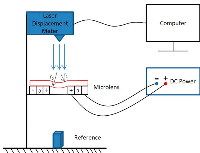
Figure 9. Schematic diagram of the focal length test process.
