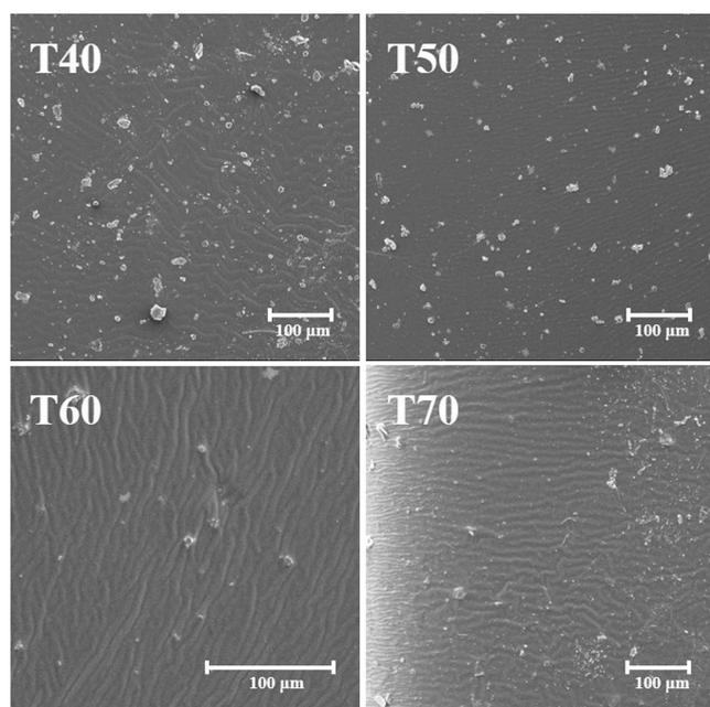
Figure 7. SEM surface test of the gels.
