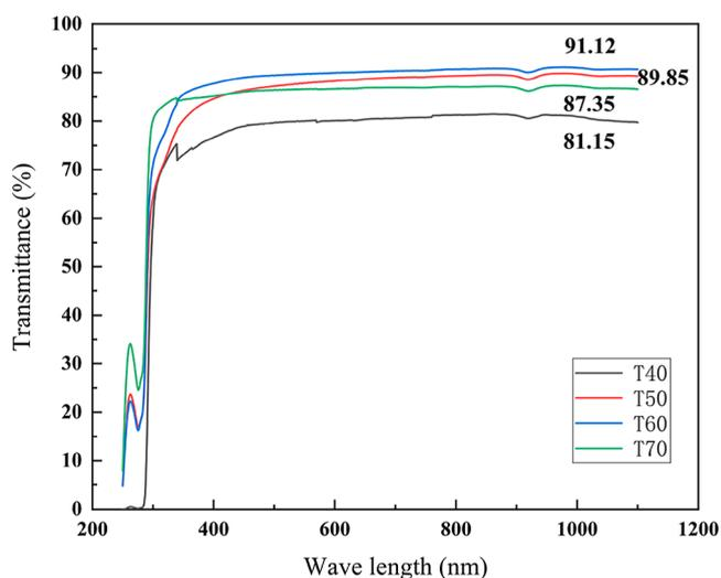
**Figure 5.** Gel light transmittance test.
