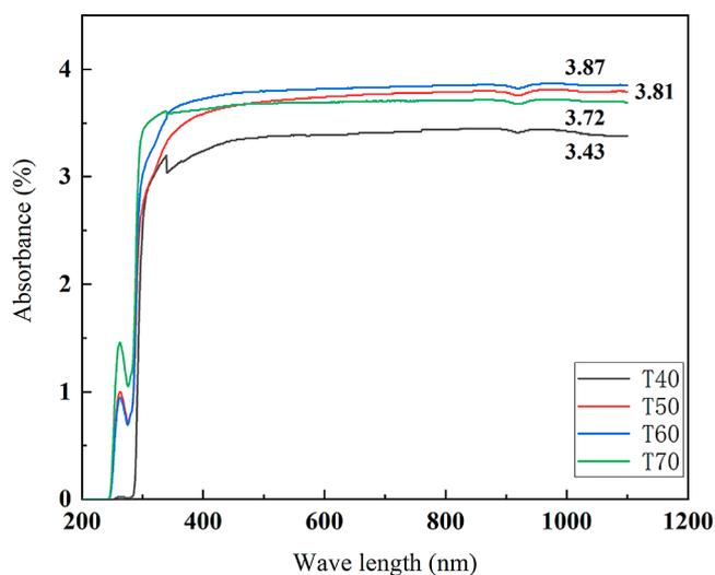
**Figure 6.** PVC gels' absorbance test.
