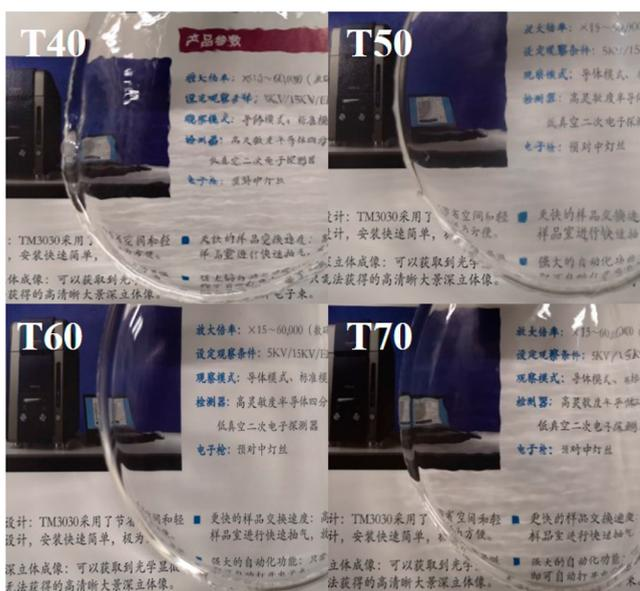
**Figure 4.** Comparison of gel transparency effects of PVC gel samples. Photograph courtesy of “Li Xudong”. Copyright 2023.
