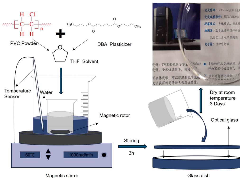
**Figure 2.** PVC gel samples' preparation process. Photograph courtesy of “Li Xudong”. Copyright 2023.
