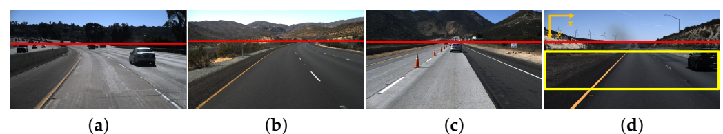
Figure 2. Red lines indicate the vanishing lines of lane markings: (a) leftward curve; (b) rightward curve; (c) downhill; and (d) uphill. The yellow rectangle is a regular ROI of the proposed method.
