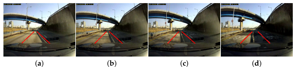
Figure 9. Sample result images of false detection in consecutive frames in the daytime sequence on KIST dataset: (a) T frame; (b) T+1 frame; (c) T+2 frame; and (d) T+3 frame.
