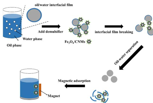
**Figure 14.** Demulsification mechanism of  $\text{Fe}_3\text{O}_4/\text{CNNs}$ .
