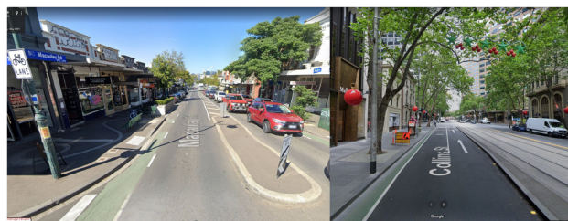
Figure 1. Google Street View screenshots showing examples of cycle lanes being ‘squeezed in’ within the City of Melbourne cycle lanes that are narrow (less than 0.6 m wide) and do not provide physical separation by a concrete curb. (left) Kensington and (right) Collins Street Melbourne.
