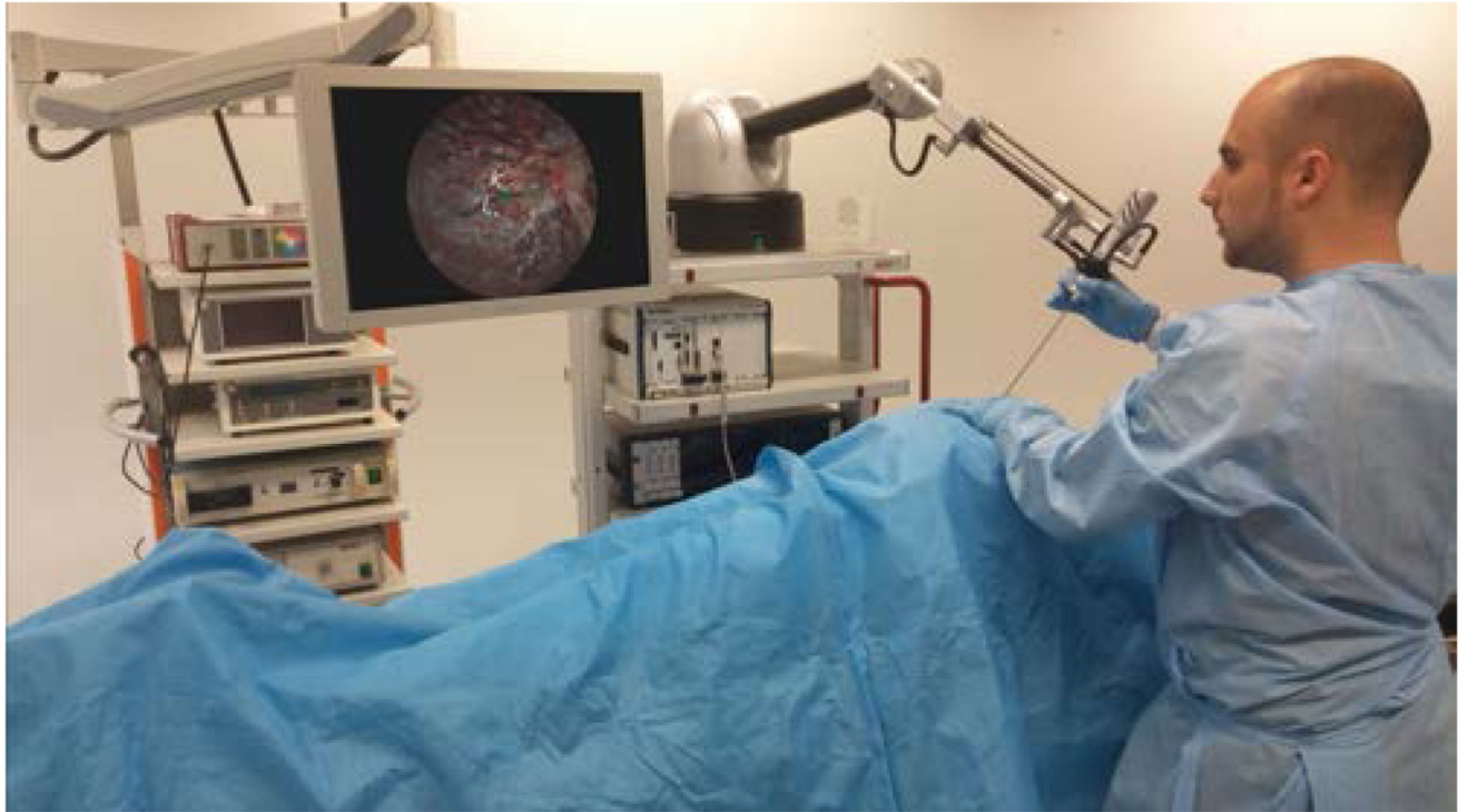
Fig. 2. Comanipulation setup for fetal surgery, with the robotic manipulator, the surgeon, and the patient.
