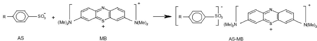
Figure 1. Mechanism of formation of ionic pair methylene blue–active substance (AS–MB) between the anionic surfactant (AS) and methylene blue (MB).
