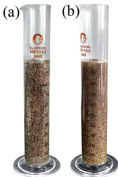
Fig. 15 Images of the proppant suspension, (a) before settling at 25 °C and (b) after settling at 65 °C over 3 h.
