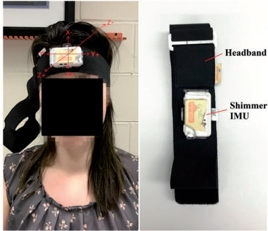
**Figure 1.** Elastic headband with one Shimmer IMU. The axis directions of the IMU are shown in the *Left*. The reference system for the head was defined as  $z+$  as anterior,  $y+$  as left and  $x-$  as superior. IMU: inertial measurement unit.
