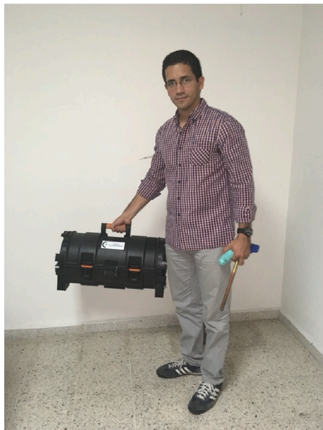
Fig. 4. The CryoPen® uses compression cooling technology instead of gas and consists of a sturdy and portable toolbox. The treatment application metal probe, held on the left hand, is detachable from the cooling unit.
