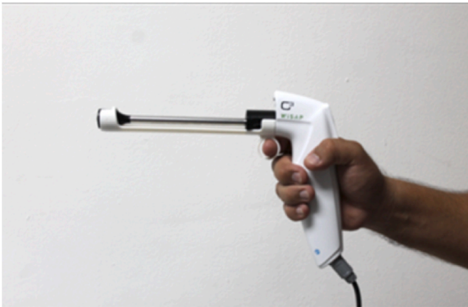
Fig. 5. The C3 WISAP portable thermal ablation device is lightweight and easy to handle. It can run on electricity or connected to a small rechargeable battery.
