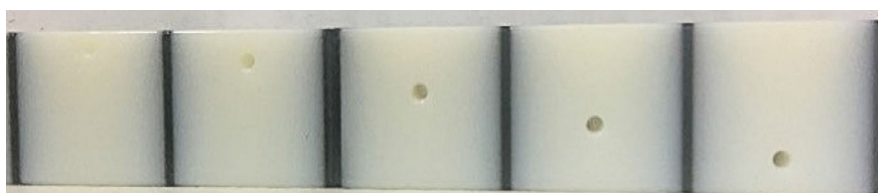
FIG. 2. 3D-printed multichannel phantom for penetration depth measurements. [Color figure can be viewed at wileyonlinelibrary.com ]
