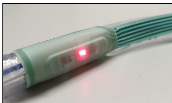
Figure 3. The ET Sensor attached to a standard adult size 7 ET Tube.
