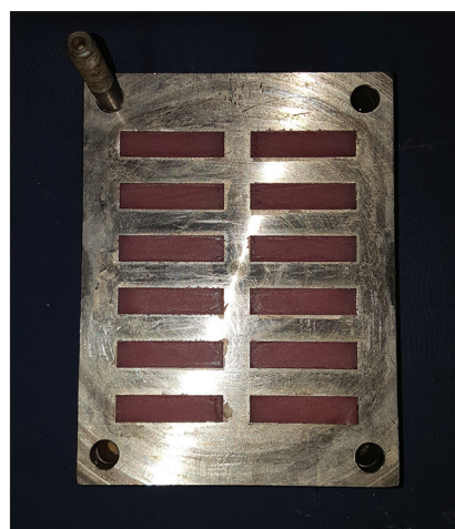
Figure 1: Packing of the acrylic resin into the special flask for preparation of the acrylic resin blocks.
