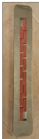
Figure 2: Preparation of the samples in a custom-made flask for the SBS test.
