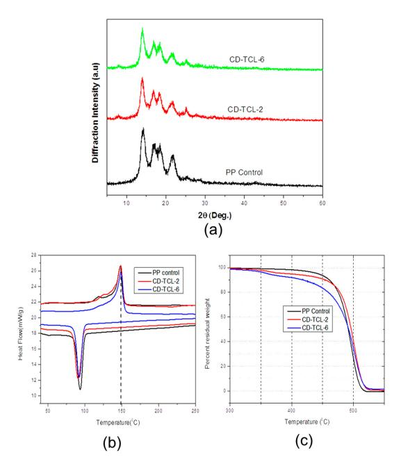
**Figure 7.** Structural and thermal properties: (a) XRD pattern of treated and untreated PP meshes; (b) DSC of PP control and modified samples; (c) TGA: percentage residual weight changes of PP control and modified samples.
