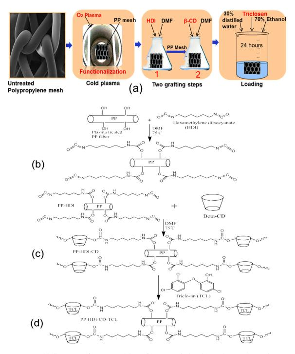
**Figure 1.** (a) Illustrations of experimental design for β-CD grafted antibacterial surgical PP meshes; Schemes (b) step-1, PP-HDI grafting; (c) step-2, PP-HDI-CD grafting; and (d) triclosan loaded meshes.
