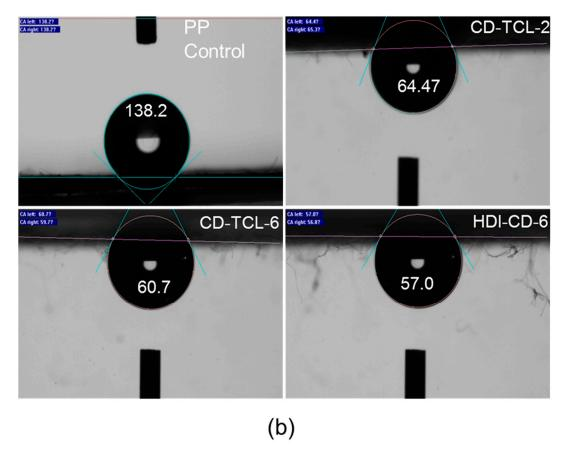
**Figure 6.** (a) Contact angles measured by sessile drop method and captive bubble (b) average contact angle drops, PP control (sessile drop), triclosan-loaded CD-TCL-2, triclosan-loaded CD-TCL-6 and CD-grafted HDI-CD-6. Data for each sample are expressed as an average of five measurements (n = 5). Statistical differences are indicated with (\*\*\*) for p < 0.001 and (\*\*) for p < 0.01.
