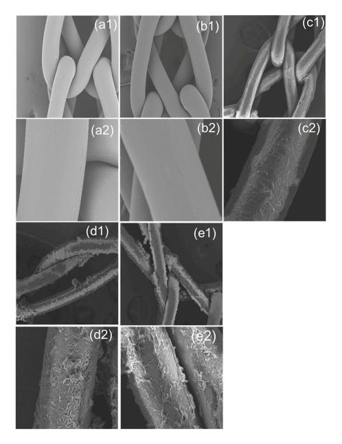
**Figure 3.** SEM micrographs; (a1,a2) PP control; (b1,b2) oxygen plasma treated; (c1,c2) HDI grafted PP-HDI-6; (d1,d2) HDI-CD-6; and (e1,e2) CD-TCL-6 (top row  $200 \times$ , bottom row  $1000 \times$ ).
