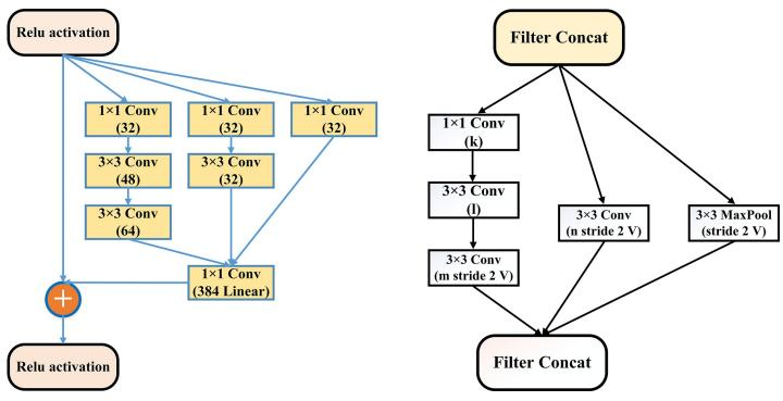
Fig 5. Illustration of CO-IRv2 (a) Inception-A module (b) Reduction-A module.
