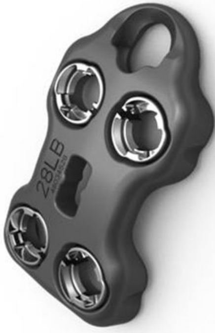
Figure 2 The anterior lumbar plate used for this study. This is fixed to the vertebral bodies through the four variables—angle holes and the integral locking rings are rotated to prevent screw back-out. The superior (fifth) hole is for optional additional compression of the intervertebral graft before placement of the two locking screws into the cranial vertebra.
