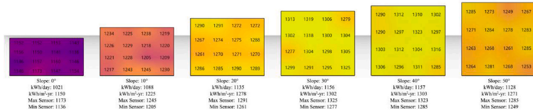
Fig. 11. Annual solar radiation received in same area panels with different slopes.
