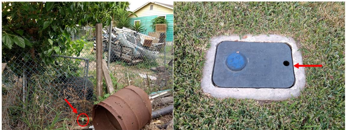
**Figure 1.** Logger placements: (left) in the open, (right) inside water meter.
