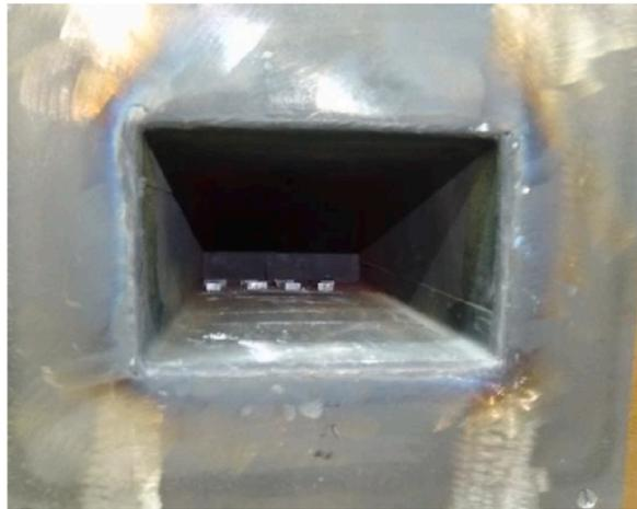
Fig. 4. Homogenization specimens in the furnace.
