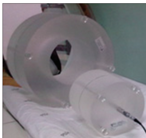
Figure 2: Computed tomography dose index head and body phantom with the pencil ion chamber inserted in the center hole of head phantom and the other holes plugged with polymethylmethacrylate pegs
