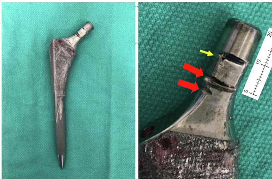
Figure 3. Notching of the femoral component neck in three distinct locations. The yellow arrow represents the first area of notching seen during the first revision. The red arrows demonstrate twin notching seen during the second revision, approximately 9 millimeters distal to the first notch.
