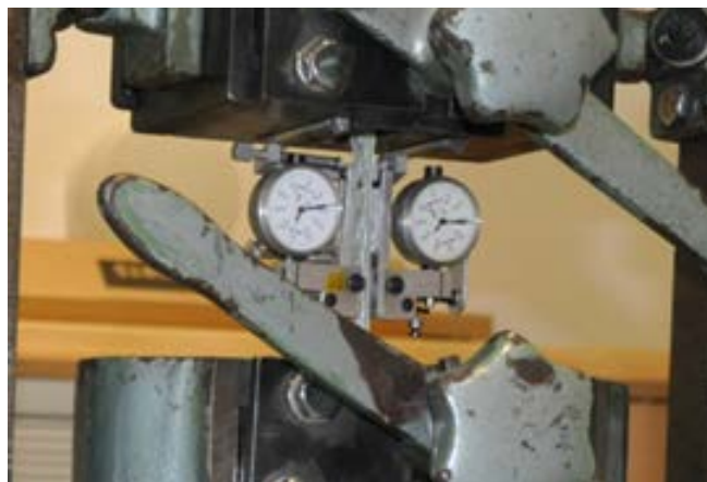
Figure 2. Specimen No. 4 during the tensile test.
