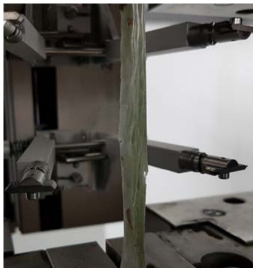
Figure 4. Ruptured specimen after static tensile test.
