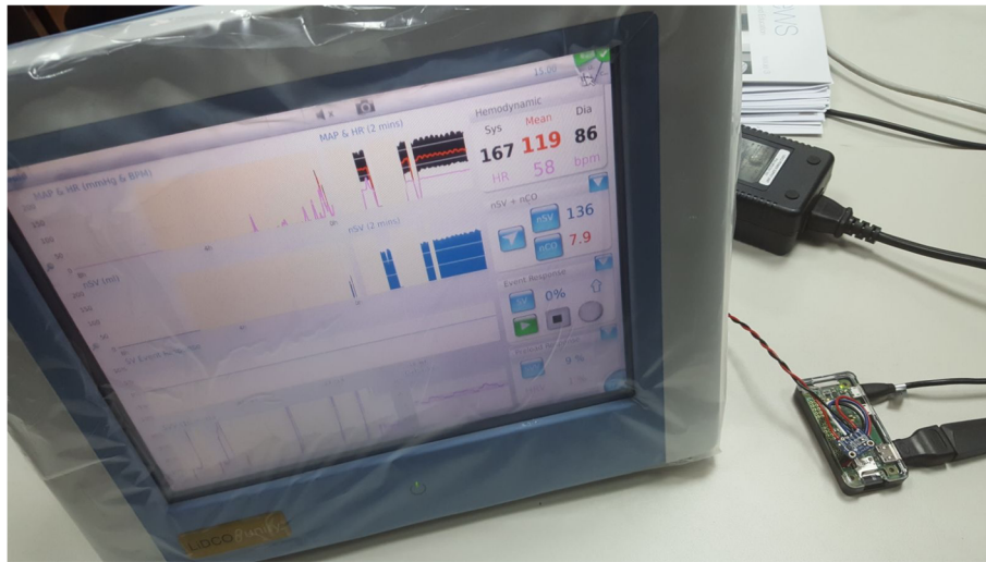
Fig. 4 Connection between the Raspberry Pi and the LiDCO monitor
