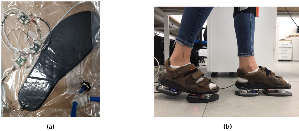
Figure 5. (a) Vacuum bag experiment. The pressure inside the bag was reduced by using a vacuum pump. (b) Sensorised shoes equipped with force/torque (FT) sensors and insoles.
