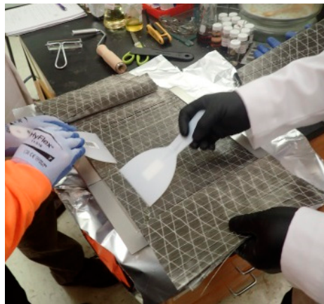
Figure 3. Saturating fibers in epoxy vinyl ester during composite preparation.
