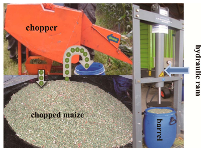
Figure 4. Setup of material preparation for Test-A with respect to ensiling process: Harvested maize was fed into a chopper. Then the chopped maize material was packed into a barrel using a hydraulic ram.
