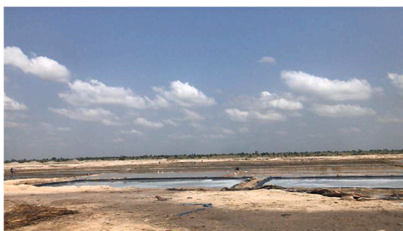
Fig. 3a. Tarpaulin lined crystallization pans in Ada West district, i.e., Songhor site, Dec 2022.
