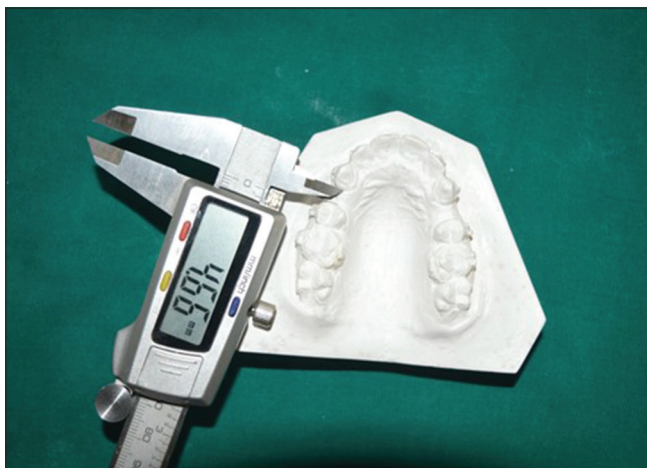
Figure 3: A digital vernier caliper was used to measure the distance between the contact points of maxillary canine and second premolar
