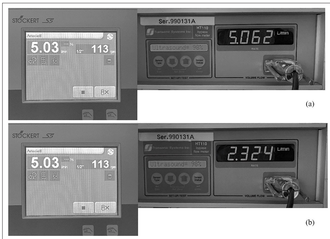
Figure 4. Photographs of the roller pump flow display (left) compared to the individually measured true flow rates (right) under normal conditions (a) and after simulated kinking of the venous tubing or volume shortage (b). Note that the roller pump flow display does not change despite changes in true flow with kinking.
