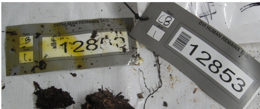
Figure 2. The link between physical evidence and digital information can be fragile: aviation fuel has damaged the printing (i.e. the label) on the left tag. (Source: Peter Ellis.)
