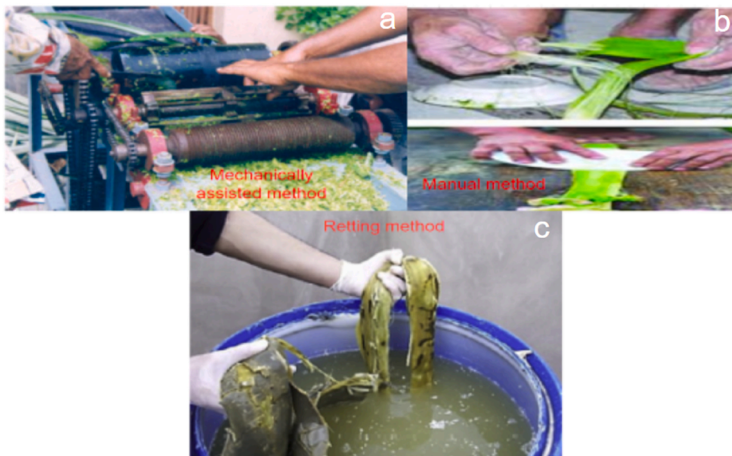
Fig. 1. Natural fiber extraction processes: (a) mechanical method (b) manual method (c) retting method [75,76].
