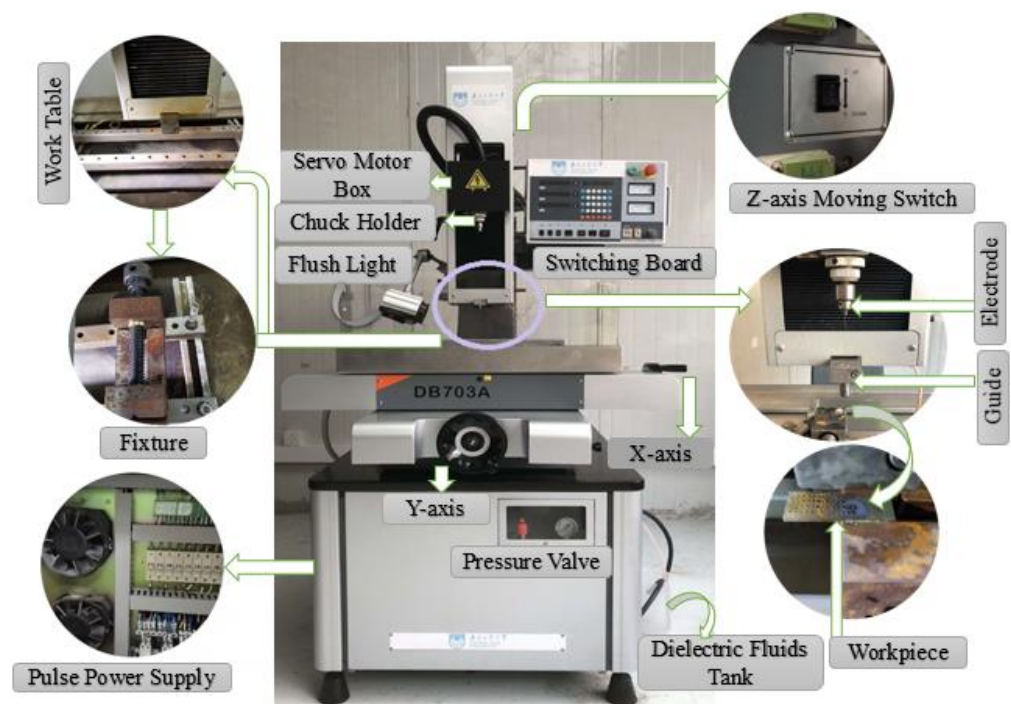
Figure 2. Photograph of the electrochemical discharge machining (ECDM) machine tool.
