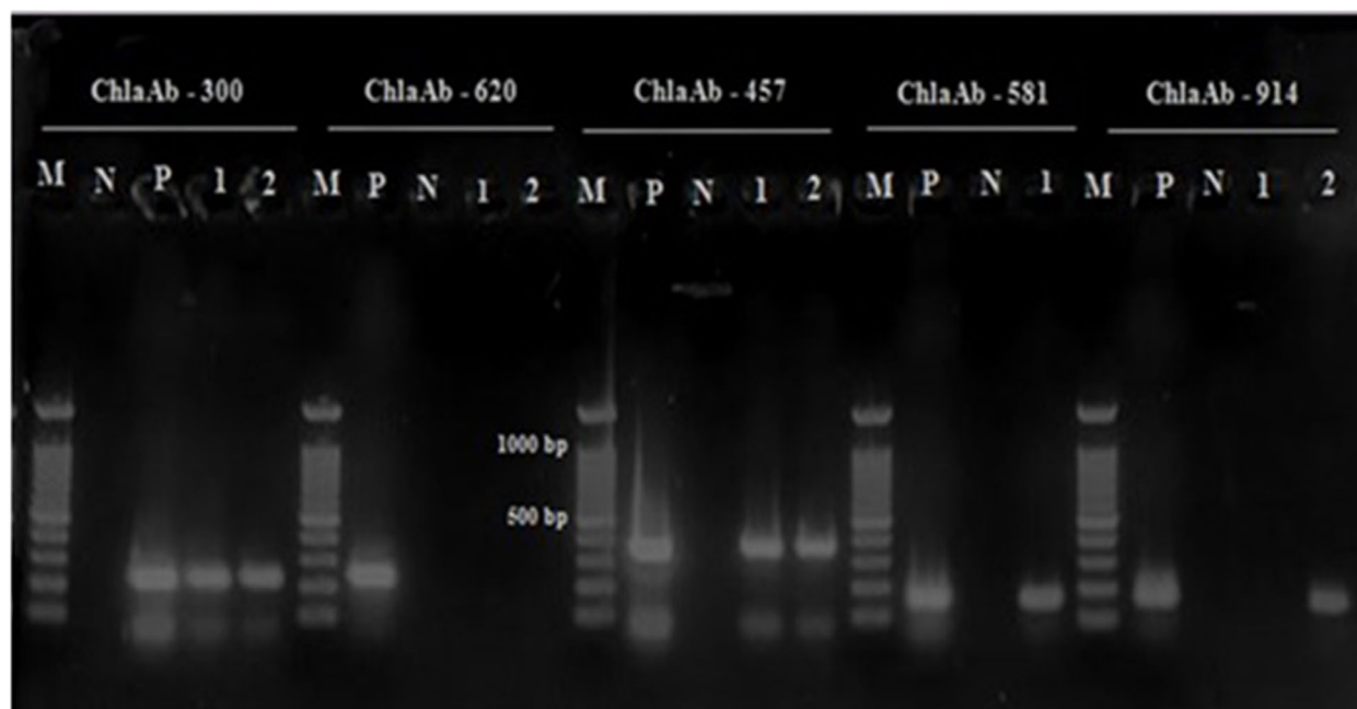
Fig. 6 MLVA profile of C. abortus in 2 studied samples. M - Molecular mass standard 100 bp ladder; N-negative control; P- C. abortus S26/3 as positive control; lines 1 and 2- tested samples
