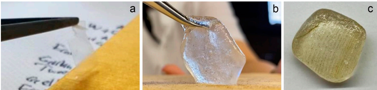
Figure 3. Images related to the application of (a) SA gel on the sweat-Western Mock-ups (WM) surface and (b) KG gel on the soiled-WM surface; (c) surface of KG gel after cleaning the soiled-East Asian Mock-ups (EAM).
