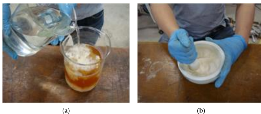
Figure 1. Making of the bio grouting material: (a) mix the microbial solution and the sodium silicate solution; and (b) make powder (calcium carbonate) in a bowl plate.
