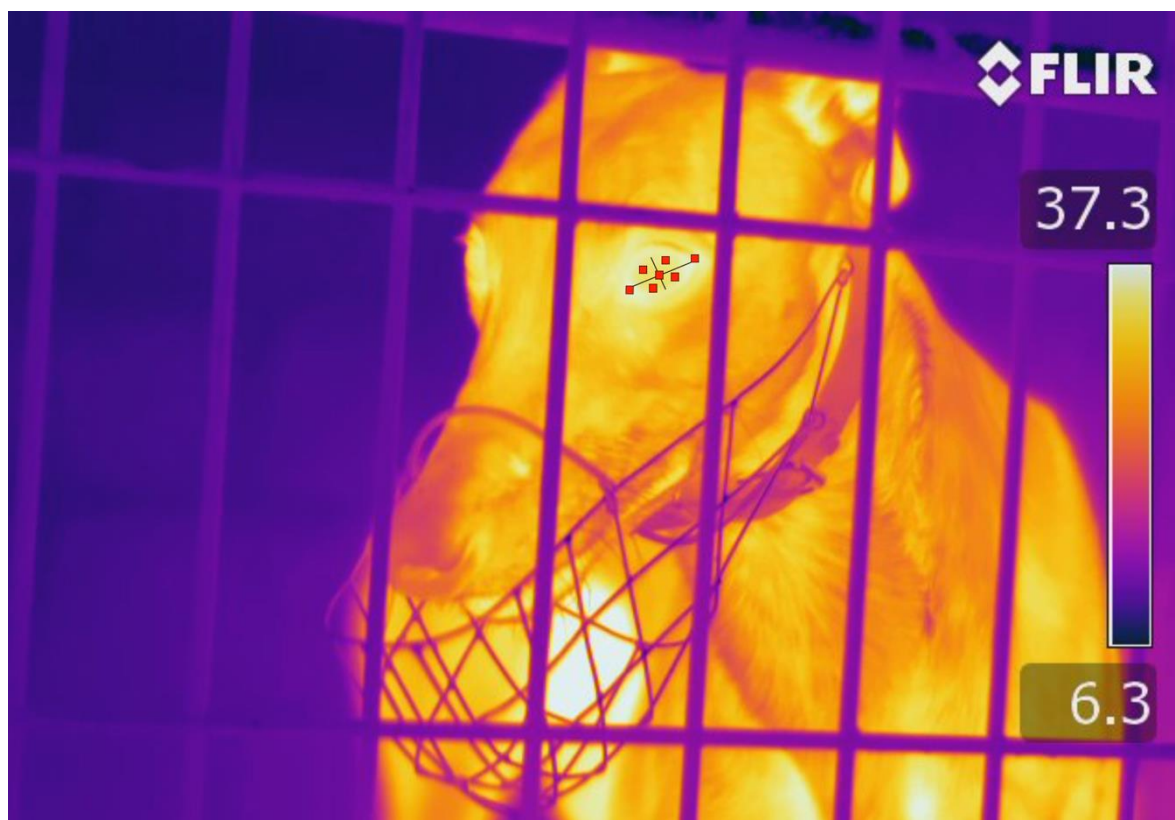
Figure 2. Infrared image of a greyhound viewed using the ResearchIR Max software. The red boxes on the left eye represent the seven locations in which the Region of Interest averages were recorded. The centre of the eye was located at the intercept of the black lines.
