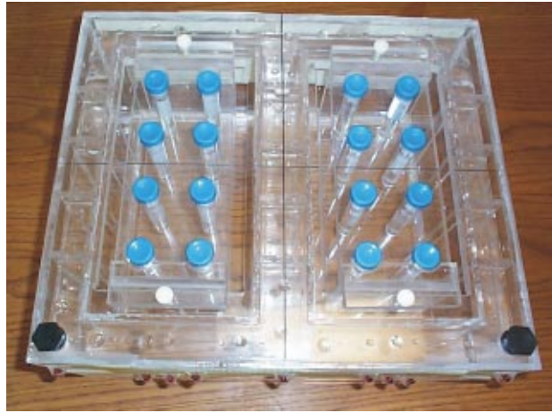
FIG. 2. (Color) A view of the phantom with the inserts in place and vials loaded for coronal imaging.
