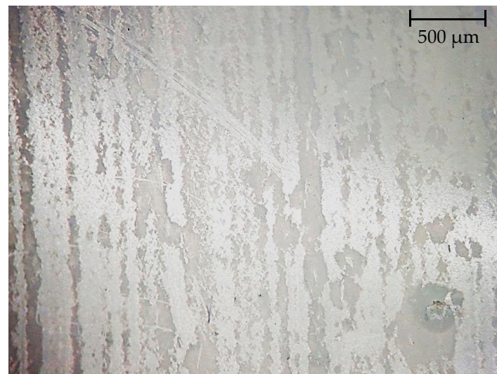
Figure 8. The inner surface of the film with betulin diffused from the film (2.3× magnification).
