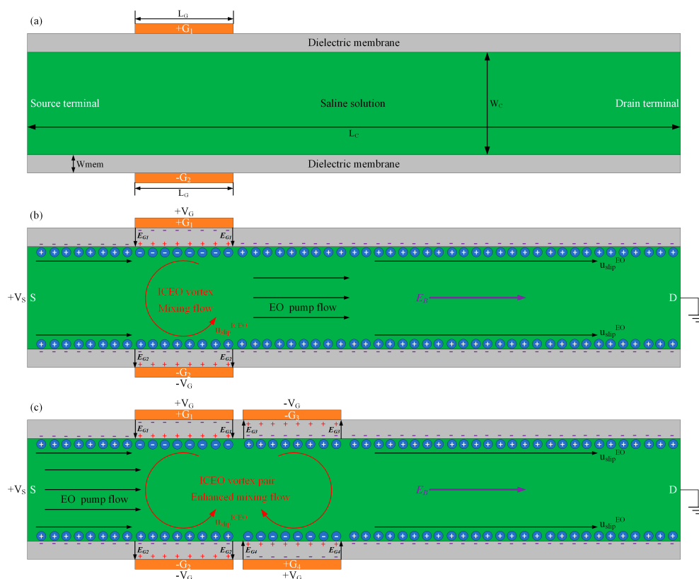
Figure 1. 2D schematic diagrams of the microfluidic device for bipolar DC field-effect electroosmosis control. (a) Geometric configuration of a bipolar DC flow field-effect-transistor (DC electroosmosis (DCEO)), in which one or several pairs of face-to-face gate (G) terminals of counter voltage polarities are embedded in a straight microchannel on the external surfaces of both sidewalls. (b,c) A vivid illustration of the physicochemical mechanism responsible for causing simultaneous sample pumping and mixing with different discrete arrangements of the external gate electrode array; (b) in the structural configuration of one pair of face-to-face oppositely-polarized gate-electrode, an individual induced-charge electroosmotic (ICEO) vortex is induced across the channel width direction next to the two G terminals; and (c) in the microfluidic device of two neighboring sets of upside-down G terminal pairs, a pair of ICEO whirlpools in reversed rotating directions is induced in the vicinity of the four external gate electrodes. Interestingly, in (c) the pair of symmetric counter-rotating ICEO micro-vortices is induced by nonlinear electroosmotic slip on the surface of polarizable membranes, within which strong electric field leakage occurs due to the action of external G terminals, and the electrokinetics-driven turbulence adds effectively to the horizontal DCEO flow component in the forward direction to achieve simultaneous pumping and mixing of electroneutral chemical analytes in microfluidics.
