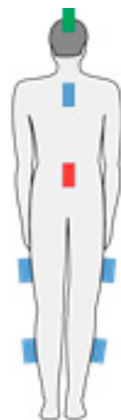
Figure 2. Placement of devices (coloured rectangles) on the body, various configurations: one-device—red; six-device—red and blue; seven-device—red, blue, and green.
