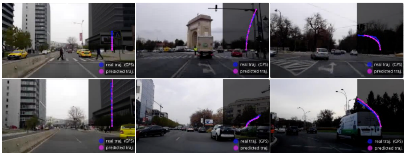
Figure 7. The trajectory predicted by the model in various traffic situations: stopping before a crosswalk (top left), accelerating when the road is clear (bottom left), before entering a roundabout (top middle), beginning to turn right (bottom middle), just before turning left (top right) and keeping left steer in a roundabout (bottom right). Notice how the trajectory, as a function of time also provides speed and acceleration information, not just spatial directions along a path. More specifically, the length of the trajectory indicates distance travelled per time. Thus, the spacing between the predicted locations in the next seven seconds are directly proportional to speed at those moments in time. The more distant the points, the faster the vehicle moves. Also, the variations in such spacing is directly related to acceleration, as the first derivative of speed with respect to time.
