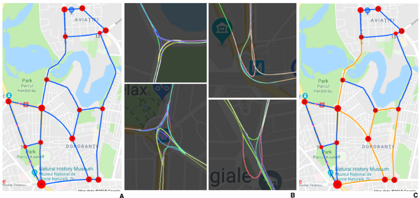
Figure 2. (A) The graph structure of the driving map. (B) Cropped sections of the analytically obtained map overlapped with the corresponding map regions from Google Maps. (C) The sub-part (orange) of the map crossed in the second phase of data collection.
