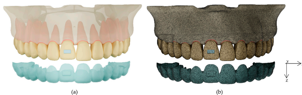
Figure 1. Maxilla model with PDL, upper teeth, clear aligner, and composite attachment: (a) 3D model and (b) finite element meshing model.
