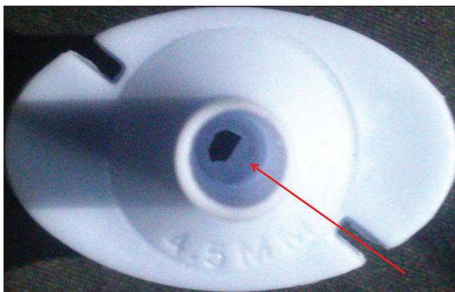
Figure 1: Distal (endotracheal) end of the defective endotracheal tube connector. Red pointed arrow is indicating a thin membranous diaphragm
