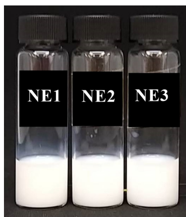
Figure 1. Chrysin nanoemulsion formulas NE1, NE2, and NE3 on the production day, pressurized at 15,000 psi for three cycles.
