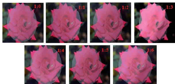
Fig. 5 Effects of different NFC : AA ratios on the transparency of NFC films.
