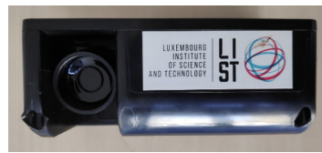
Figure 7. Brighterbins ultrasonic sensor ( L=130\text{mm} , W=70\text{mm} , H=53\text{mm} ).
