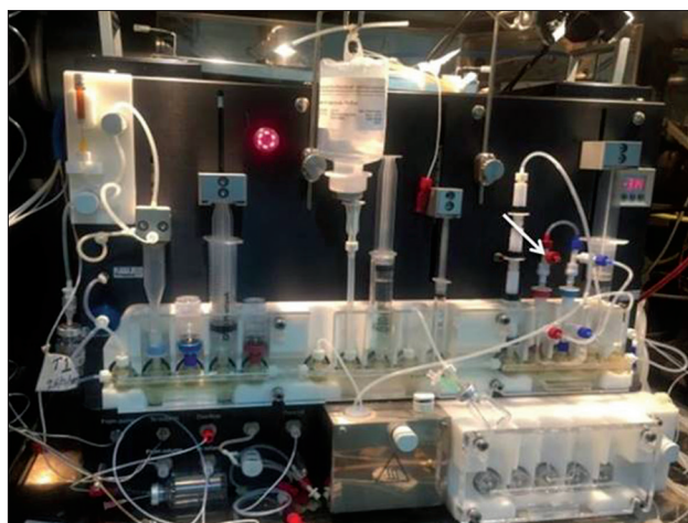
Figure 5: Leakage in line (with arrow) connecting C-18 cartridge due to overtightened check valves into the C-18 cartridge and thus leading to failure of synthesis
