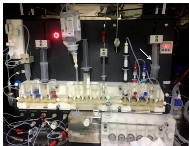
Figure 4: Deformed right syringe (with arrow) due to blockage of CM cartridge resulting in failure of synthesis
