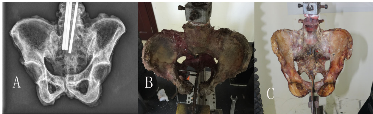
Fig. 2 a X-ray image of the pelvic specimen before the experiment. b, c Restricted hemipelvis model and unrestricted hemipelvis model, respectively
