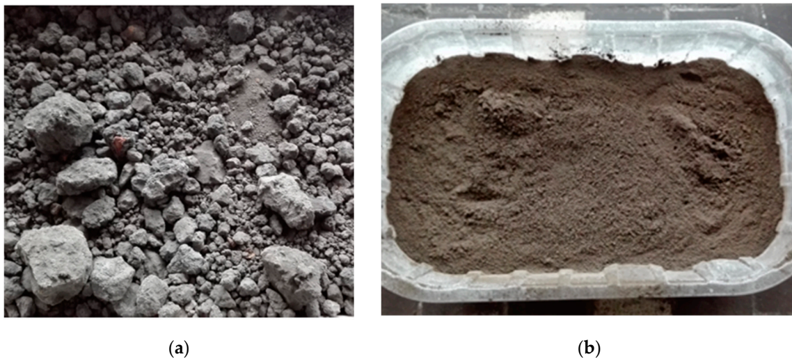
Figure 2. Metallurgical sludge waste used in research (a) unprocessed, (b) oven dried, ground.
